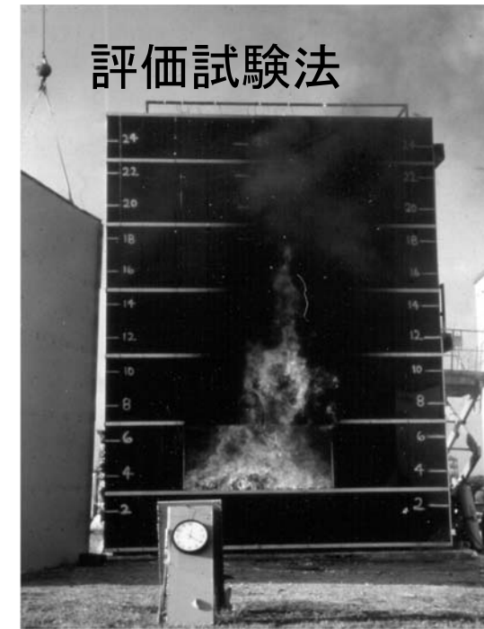
UBC26-4 Multi-story fire evaluation test
